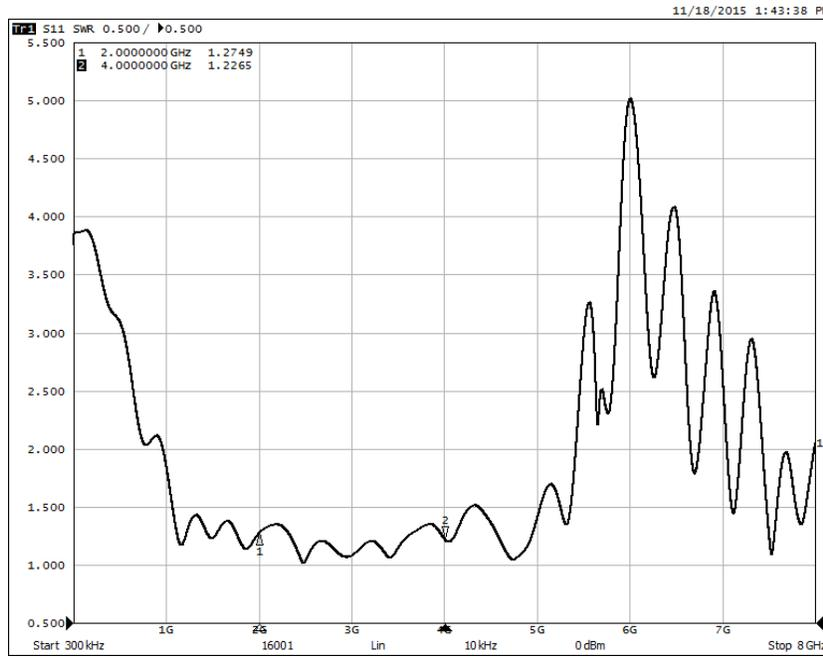
From the measurement results, we can see that the input VSWR, through the operating frequency, is always better than 1.4:1 and the transmission coefficient is about -6.4 dB for each output port. Therefore, our multipoint testing system with RF switch is providing us a good measurement result that agrees with the datasheet.
